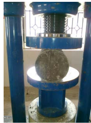
Fig. 3 Test Setup for Split Tensile Strength
